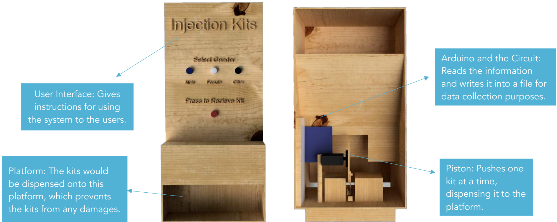
Fig 2*: The Piston Dispenser User Interface Fig 3*: Piston Dispenser Inside
