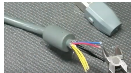
Figure 12: Xbox Power Supply - Wires Exposed
